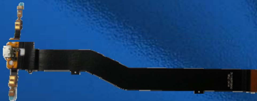
4L HDI+copper fill for USB
