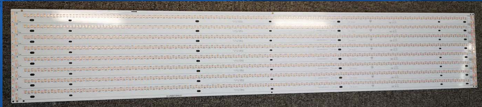
LED FR-4 PCB---2 layer 1137.9mm x 215.9mm
